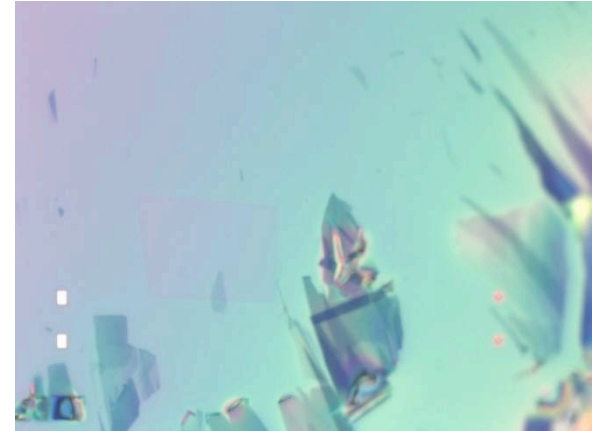
Fig. 1: Graphene flake, beneath a layer of PMMA. A square region exposed during e-beam lithography is visible (50x)
